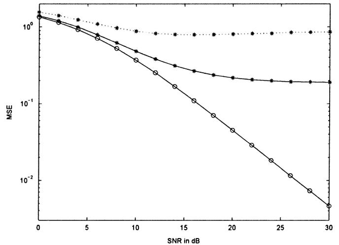
Fig. 5. MMSE using the true channel (“-o-”) and expectation of the MSEs using the channel estimate for  $\rho = 0.99$  (“-\*”) and for  $\rho = 0.9$  (dotted line).
