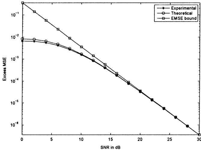
Fig. 7. Experimentally computed EMSE, theoretical second-order approximation (44), and high-SNR approximation (47) for the case of noise SOS estimation errors.
