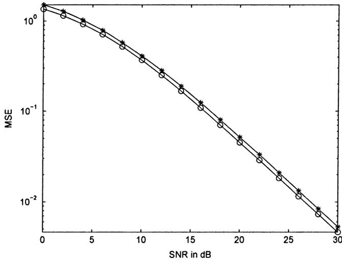
Fig. 2. MMSE using the true channel (“-o-”) and expectation of the MSEs using the channel estimate (“-\*”).
