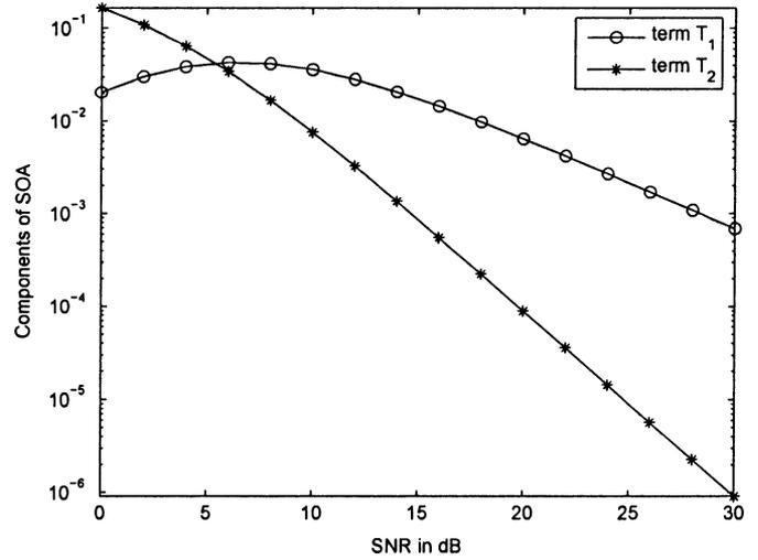
Fig. 4. Terms  $T_1$  and  $T_2$  of the EMSE second-order approximation (26) for the case of channel estimation errors.
