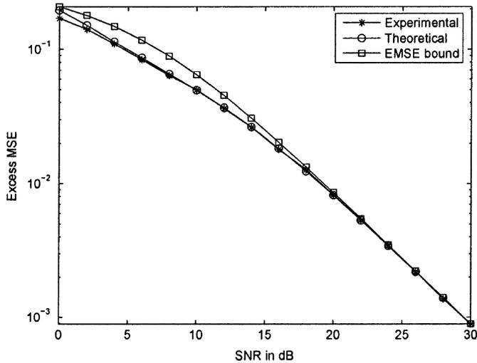
Fig. 3. Experimentally computed EMSE, theoretical second-order approximation (26), and high-SNR approximation (36) for the case of channel estimation errors.
