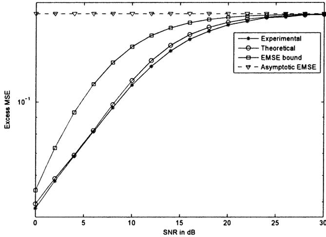
Fig. 6. Experimentally computed EMSE, theoretical second-order approximation (26), high-SNR approximation (38) and asymptotic EMSE value (39) for channel time variations ( $\rho = 0.99$ ).
