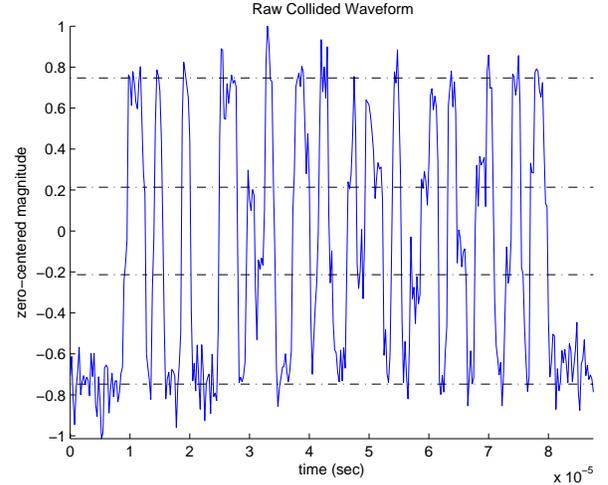
(b) Zero-centered magnitude of the received waveform for two collided FM0 tags.
