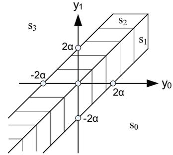
Fig. 5. Decision areas for each pair of measurements in memory-assisted detection.
