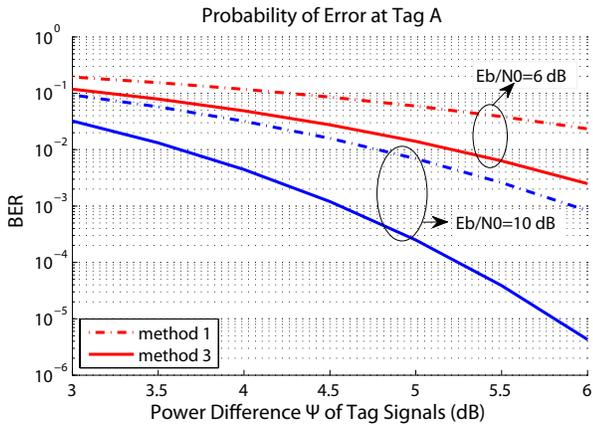
Fig. 9. BER at tag A only vs tag power ratio  $\Psi$  (fixed SNR).
