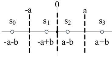
Fig. 3. The two-tag, nonuniform signal constellation with decision areas (marked with intermittent lines) based on the minimum distance rule.
