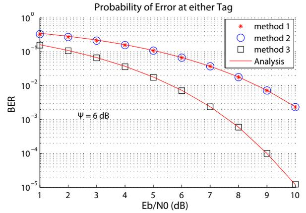
Fig. 6. BER at either tag vs SNR (fixed  $\Psi = 6$  dB).
