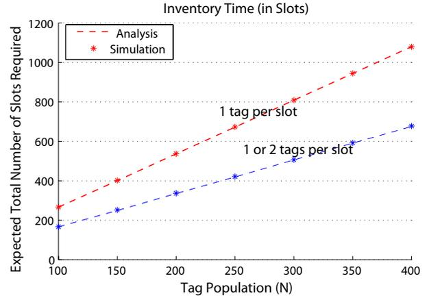
Fig. 10. Total number of required slots in framed Aloha as a function of tag population for different types of "collision".
