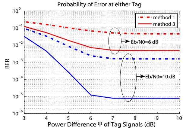
Fig. 7. BER at either tag vs tag power ratio  $\Psi$  (fixed SNR).
