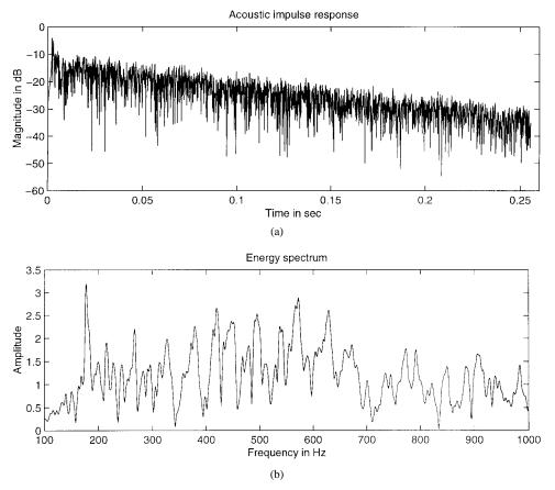
Fig. 2. (a) Magnitude of acoustic impulse response in decibel scale. (b) Energy spectrum of acoustic impulse response (frequency interval 100-1000 Hz).
