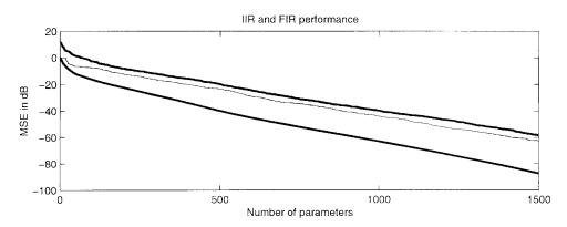
Fig. 3. Performance levels for IIR and FIR models. Thick lines: Upper and lower mean square error bounds for IIR models. Thin line: Minimum mean square error for FIR models.
