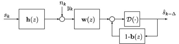
Fig. 1. Channel model and MMSE–DFE.
