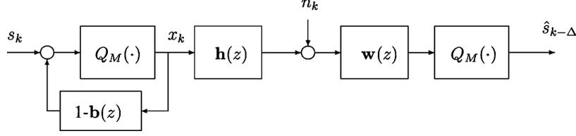
Fig. 2. TH precoding.
