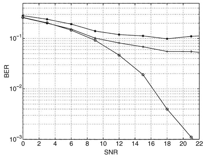
Fig. 6. BER versus SNR for MMSE-DFE (o-), robust TH precoder (+-), and conventional TH precoder (\*-), for  $\rho = 0.85$ .
