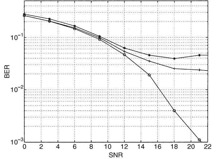
Fig. 5. BER versus SNR for MMSE-DFE (o-), robust TH precoder (+), and conventional TH precoder (\*-), for  $\rho = 0.94$ .
