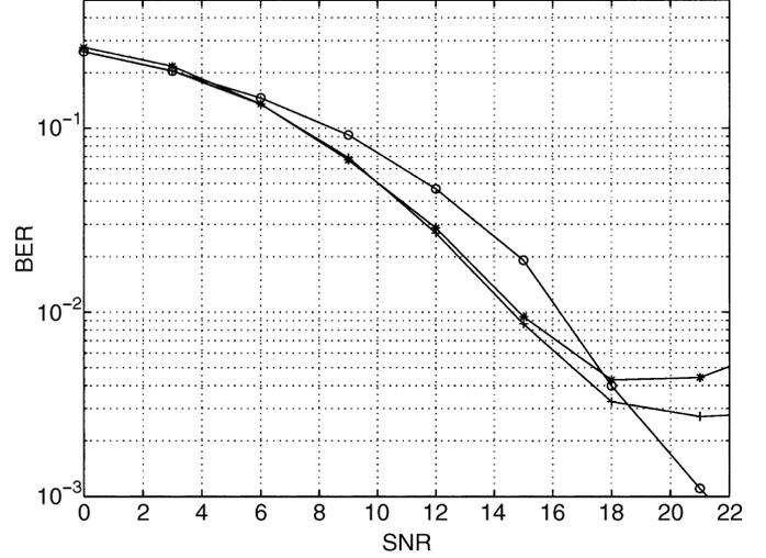
Fig. 4. BER versus SNR for MMSE-DFE (o-), robust TH precoder (+), and conventional TH precoder (\*-), for  $\rho = 0.99$ .
