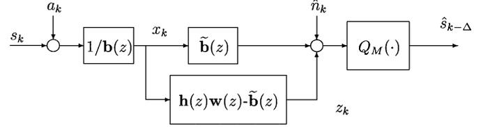
Fig. 3. TH precoding (equivalent structure).
